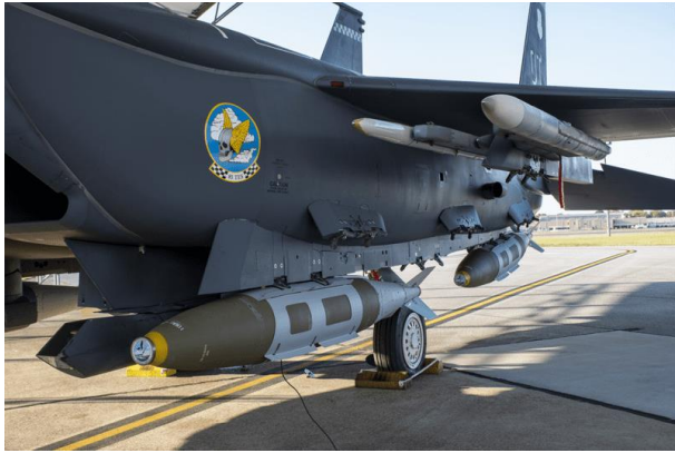
An F-15E Strike Eagle at Eglin Air Force Base, Florida, with modified 2,000-pound GBU-31 Joint Direct Attack Munitions as part of the second test in the QUICKSINK Joint Capability Technology Demonstration. (U.S. Air Force photo / 1st Lt Lindsey Heflin)
